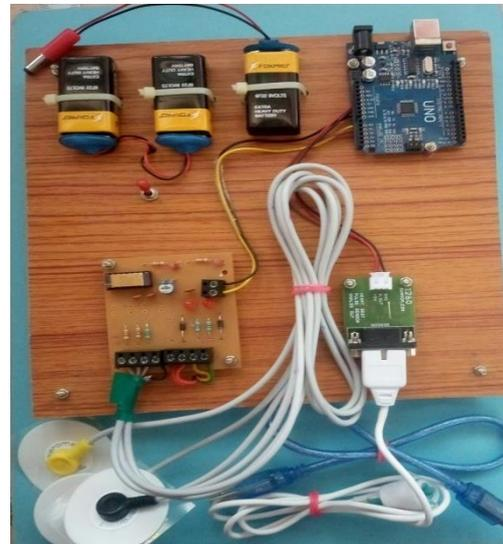
Fig 7. Real time monitoring of ECG signal and pulse rate
