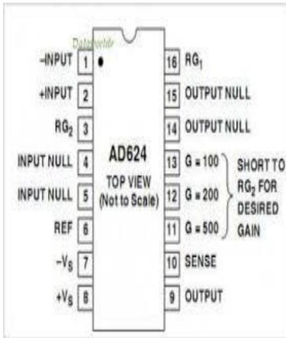
Fig 5. pin diagram of AD624
