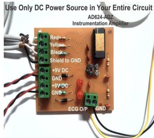
Fig 4. Instrumentation amplifier
