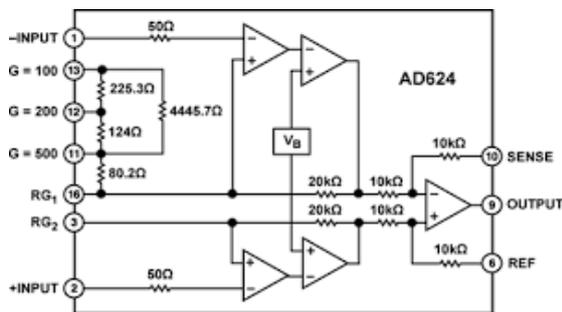
Fig 6. Circuit diagram of AD624
